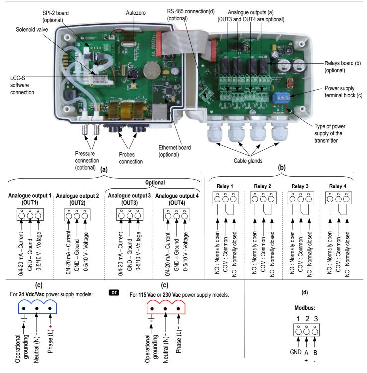
This connection must be made by a formed and qualified technician. Whilst making the connection, the transmitter must not be energized. The presence of a switch or a circuit breaker upstream the device is compulsory.
